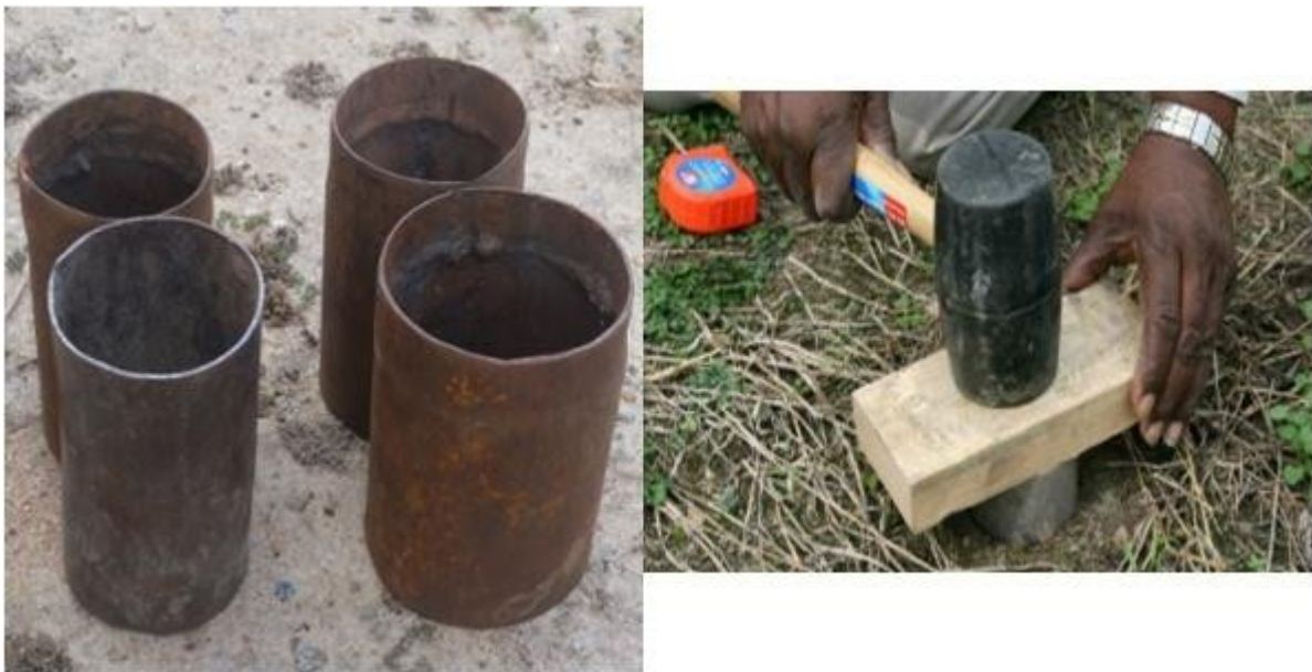
Figure 4. the core samplers used in this study and a part of the procedure for sample collection.
